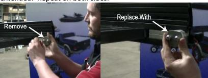
2.4 Add hardware onto the TRUCKBOSS deck. -- On each side, four 5/16 by 3/4" bolts will be added to the surface of the deck and two knobs with 1" carriage bolts will be added to the deck sides. The two 3/4" carriage bolts should be added into each of the two rear capture channels on each side. The knobs should be added into the lower of the two capture channels on the each of the sides.
