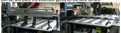
2.14.5 Slide out the extension side. Line up a single bolt (in TRUCKBOSS side) with the middle hole in the extension side. Secure with knob. Secure spare bolt on TRUCKBOSS side with a knob. The spare bolt and knob can be attached to the surface bracket. Repeat that process for the other side. Close the TRUCKBOSS sides. Ready for transport.
