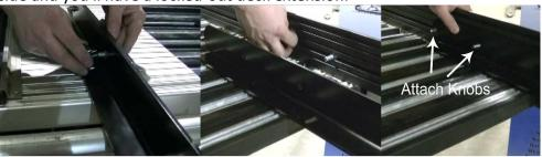
2.13 With the deck extension now locked in the out position the sides can be shut.
